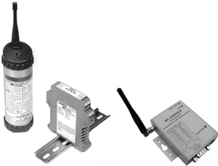
FIGURE 7.13 Some types of compact industrial radio transmitter/receiver devices, with service area up to 1 km.
