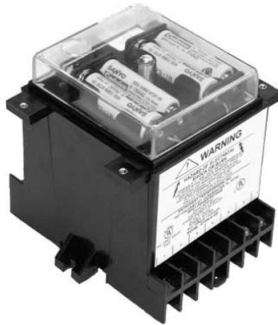
FIGURE 6.1 One of the modern capacitor trip units providing accumulation and long storage of energy for a feed of trip coil of circuit breaker with absence of an auxiliary voltage.
