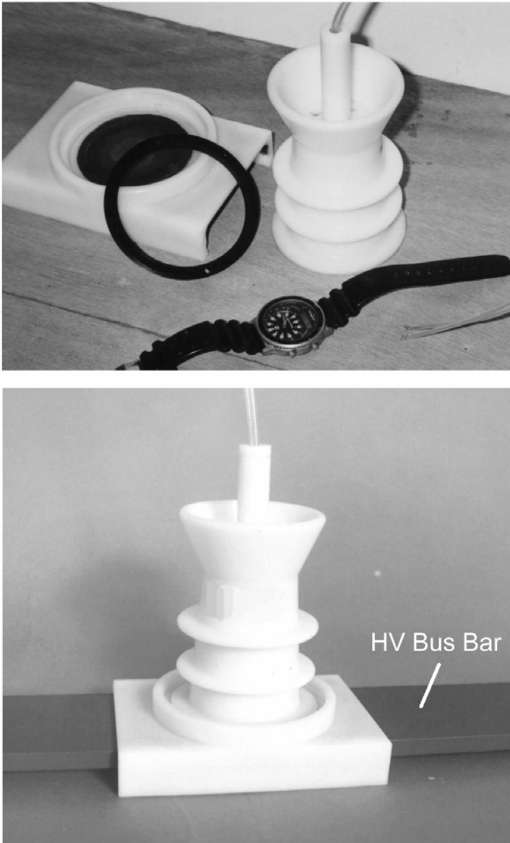
FIGURE 3.10 Installation of RG-24-bus device on a high voltage bus bar.
