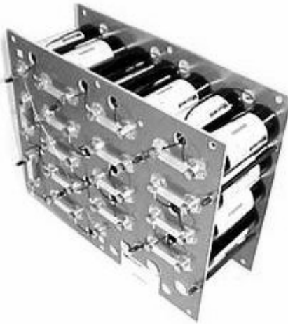
FIGURE 6.6 Internal design of high-voltage (ten voltages) supercapacitor, assembled from number of low-voltage elements.
