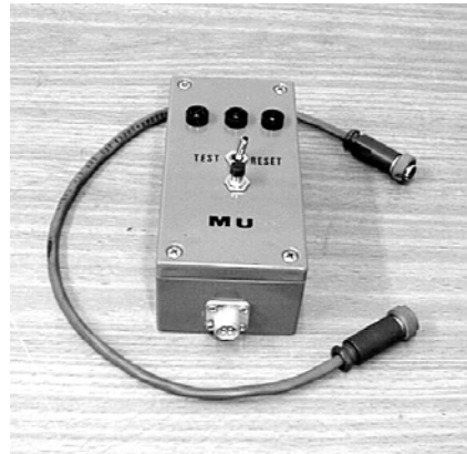
FIGURE 7.25 Manual unit of GCFI system.
